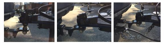
(1) crank the tongue of the trailer jack until the hitch coupler is raised enough to clear the tow vehicle;
