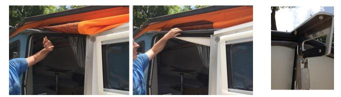
10. Walk around the trailer and tuck in any orange fabric you might see. At every tent window location feel with your fingers to make sure the wooden toggle is inboard of the skeleton.
