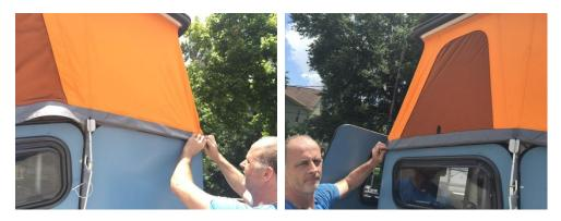
6. Pull the tent side front down to minimize wrinkles and attach the lower Velcro edge to the corner. Repeat for other side.
