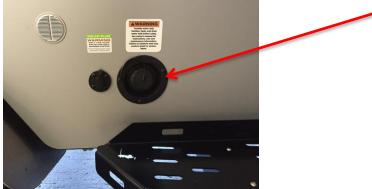
(2) Connect one end of a potable water transfer hose to a water supply, turn on the water supply and let the water run until it is clean and clear; (3) Turn off the water supply, and place the other end of the transfer hose into the fresh water inlet located on the side of the trailer; (4) Turn on the water supply and fill the tank until tank is full. Avoid overflowing tank as this can fill the vent tube with water. If the vent tube gets full of water the tank can become difficult to fill.
