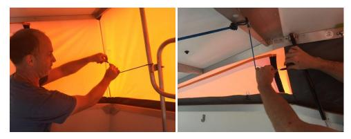
1. inside the trailer remove the 5 bungees that provide tension to the tent side. 3 are over the kitchen counter. 2 are at the mid-point of the tent side above the hold down latches.
