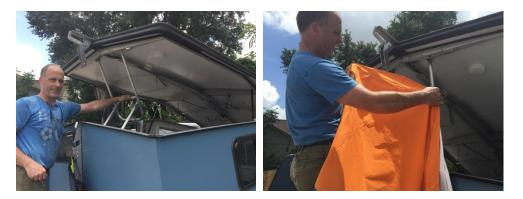
1. Open your Cricket roof partially. Do NOT push that front bracket all the way up. Find the top center of your tent side. The grey edge is the bottom. Stand on the tongue, the toolbox or a step ladder.
