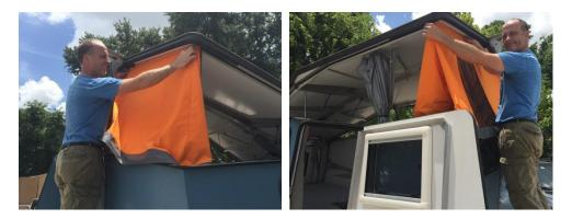
2. Lay the two long trailing ends of the tent side on the kitchen counter on either side of the bracket. Take the center and press it to the Velcro along the top edge of the Cricket. Keep one hand at the center and run the Velcro out to the corner, pressing Velcro to Velcro. Repeat with other side.
