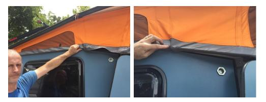
8. Attach this last foot or so from the front to the rear. There may or may not be a small fold that needs folding here (depends on model year and tent side). Make a rear facing fold in line with the seam in the tent side. Repeat on other side.
