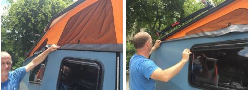
7. Attach the lower Velcro from the front corner back to the door post. Pull down slightly to remove wrinkles. STOP. Attach the lower Velcro from the rear tail forward to a point just above the forward corner of the large window where the skeleton bumps out toward the door post. This leaves about one foot unattached.
