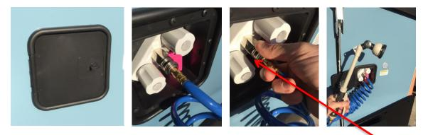
To remove the hose after use push the nickel ring in (towards trailer) and the brass end should pop out. Hose off your head, your feet, your dog, etc. Use the privacy enclosure for a full on shower.
