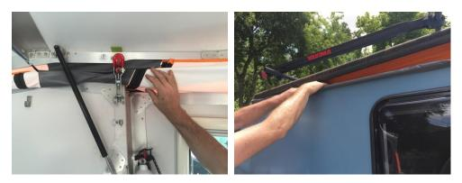
9. If latching the tent side down for driving or storage - pull down the roof and loosely catch the J-hook so that the roof is about 3 or 4 inches from being pulled all the way down. Exit the trailer.
