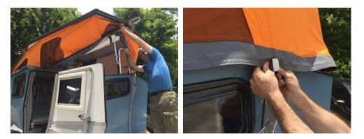
5. Go back to the front of the trailer, inside or out, and push the roof bracket all the way up. Find the center bottom of the tent side (there is a small slit in the grey there) and pull it down to either side of the guide in the lower skeleton.
