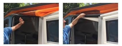
4. At the center front exterior push the exterior latch in place – push it until the pin is past the spring latch. Make sure that the roof is centered within guides. Some of you will be able to insert the clevis pin at this point. If it is too much wrestling wait on this til after step 5!
