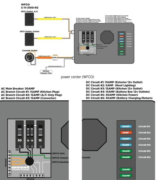
WARNING: NEVER REPLACE INSTALLED CIRCUIT BREAKERS OR FUSES WITH CIRCUIT BREAKERS OR FUSES OF HIGHER AMPERAGE RATING THAN THOSE ORIGINALLY INSTALLED. THIS COULD OVERHEAT THE WIRING AND START A FIRE.
