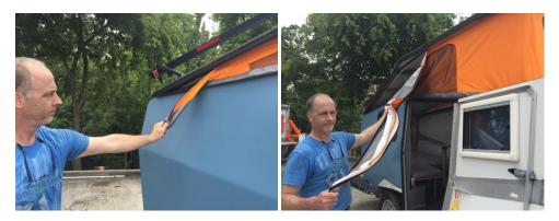
2. outside the trailer, go to the rear of the trailer and grab the tail of the tent, pull that out perpendicular to the side of the trailer.
