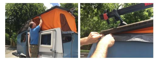
4. Move to one side of the trailer and continue attaching the top edge of Velcro. Depending on your height you may want a step stool or to use one arm to lower the roof a bit more as you work to the rear. When you get to the tail you will need to use your fingers to shove the tent side in to adhere the Velcro. This is easier the lower the roof is. The very end of the tail should pull out the rear of the roof (just barely). Repeat on other side of trailer.
