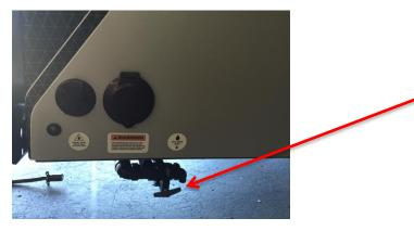
Hand shower / hose ... your Cricket TREK and CAMP have a shower! Located on the front driver's side is a black door behind which hides a hot and cold water valve and a Quick Disconnect (QD) valve to insert the blue coiled hose. The brass end on the hose simply pushes into the QD receptacle – a click will indicate it is secure.
