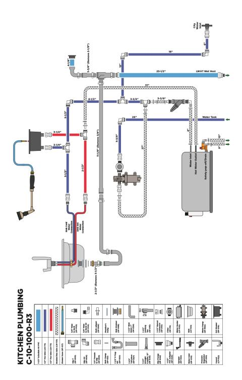
*overview* .... your trailer's fresh water system is a vital part of your traveling life while on the road. Your CAMP or TREK trailer is equipped with a dual supply water system: (1) the demand fresh water system operates from the trailer's supply tank and water pump; and (2) the "city water" hookup allows you to connect to a pressurized external water system at a campground.
