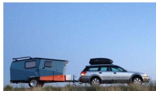
proper ~10 to 15% of loaded trailer on tongue
