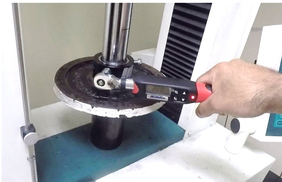
Figure 13. Installation of the Mack Clamps using a torque wrench
