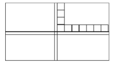
If it is decided to have the center row of tiles straddle either or both of the center lines, additional guidelines should be snapped on the floor 1/2 tiles width on one side of either or both center lines as required. (See Figure 2)
