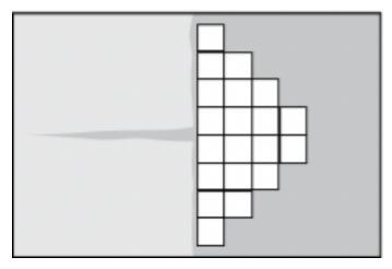
Spread the adhesive over one-half the area and after it is ready, start laying tile from the right angle formed in the center of the room by center lines. Lay toward the two corners of the room as shown. Always refer to your guide lines as you progress with laying so that a mistake can be corrected before it
