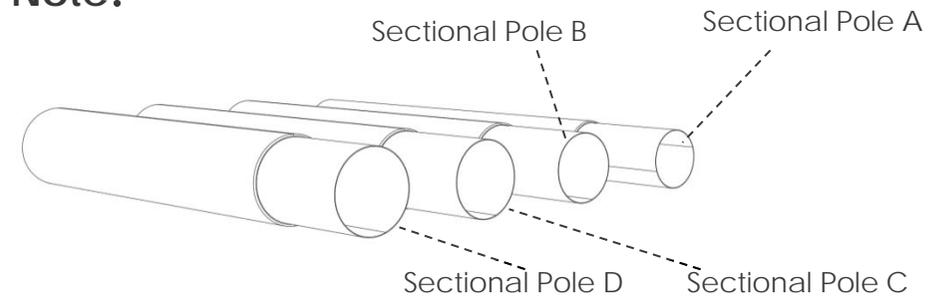
1. The diameters of the protruding part of the sectional pole A, B, C and D slightly increase in order. Please differentiate these poles correctly.
