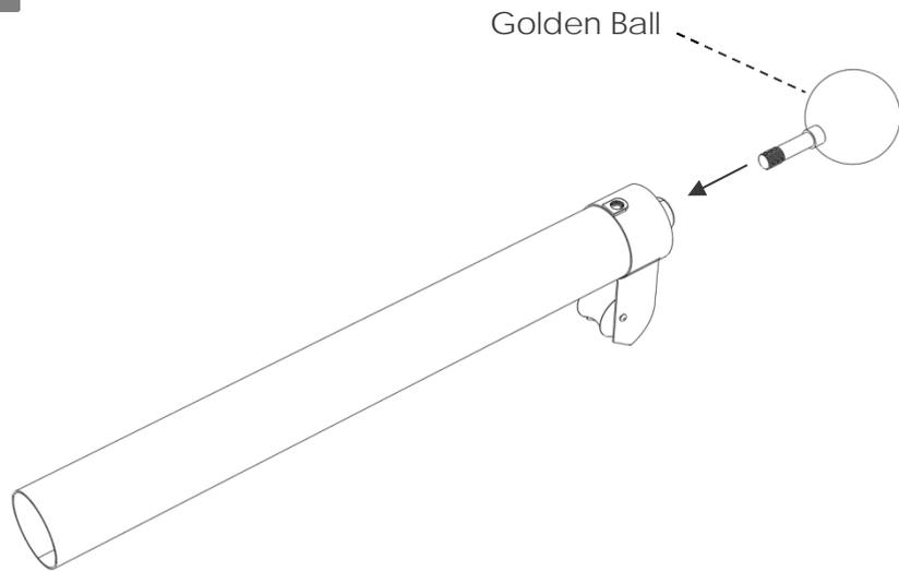
Install the golden ball onto the rotating collar.
