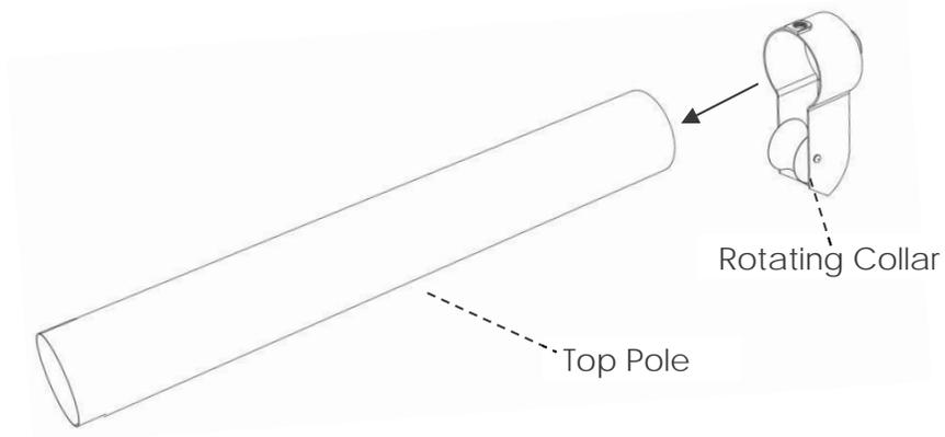
Install the rotating collar onto the top pole.
