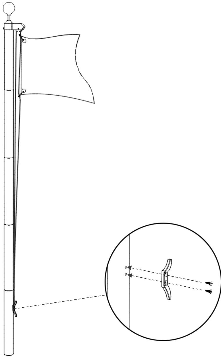
Use two screws to install the rope winder onto the pole. Bind the two ends of the rope together. After that, wind the rope on the rope winder.
