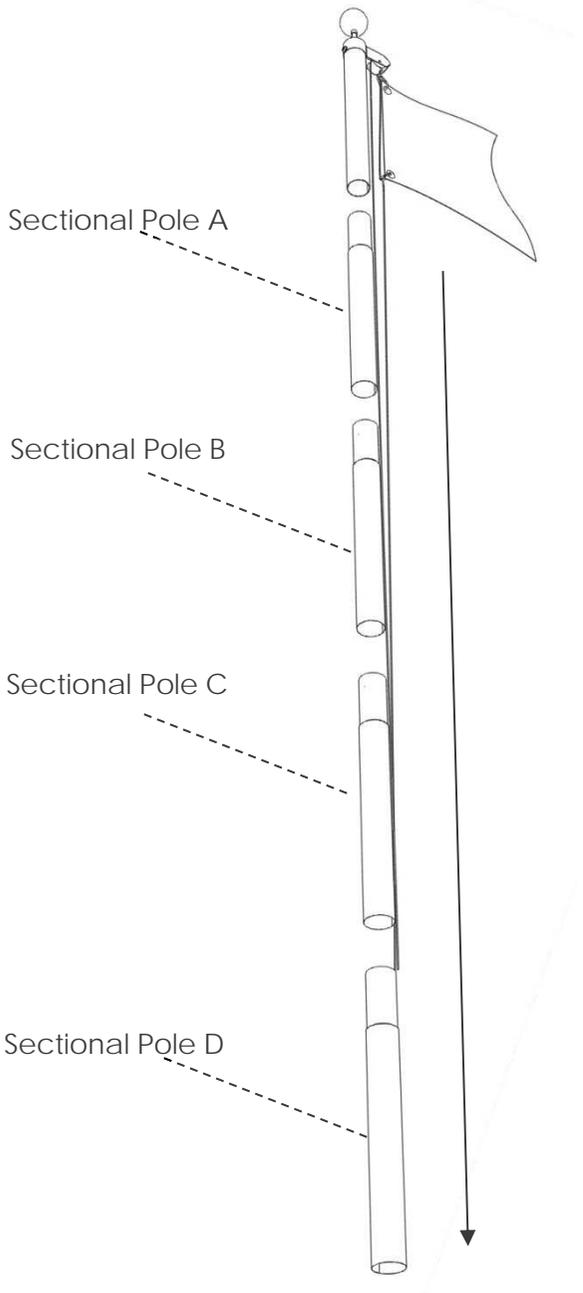
Connect the sectional poles together as shown above.
