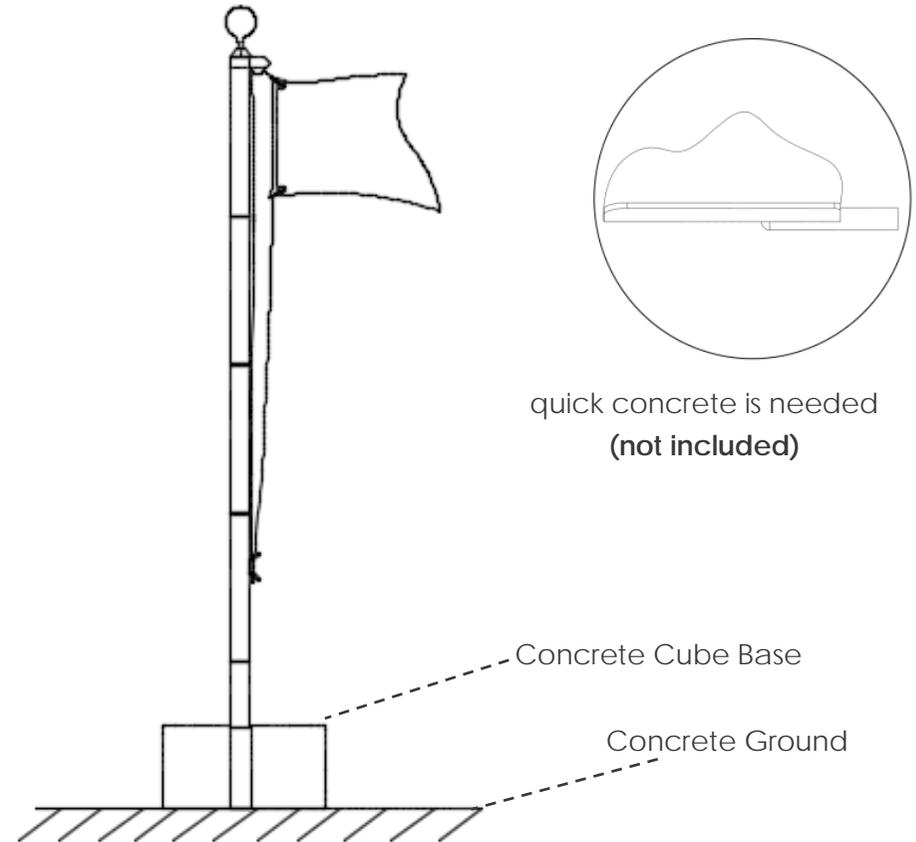
You can use quick concrete to form a concrete cube base to secure up the flag pole. **(Customer needs to buy quick concrete additionally.)**
