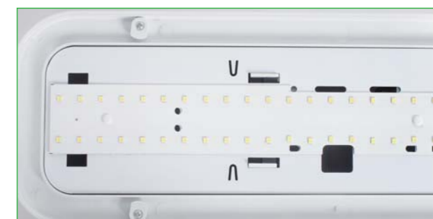
Option 2: LED SMD type High lumen efficiency 100lm/w
