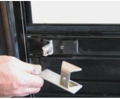
The bracket is removed from below.
