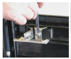
Pull the cover to the tailgate and open the tailgate. Remove lock bracket bolt (10mm) from below the lock.
