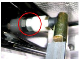
Use plastic tie to secure each linkage to the shaft so they do not get caught in the cover when rolling out of the spiral.
