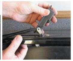
The lock is removed from the top. Lift the lock up and slide it over to the passenger side of the lock opening to remove. The lock may need to be partially open and turned at a right angle for clearance when removing lock.
