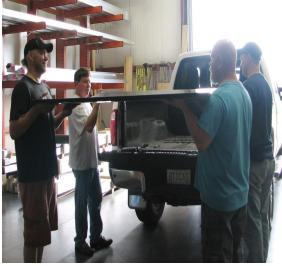
Hold the rolling cover up slightly as it is slid into the rails. Take it slow and watch out for your fingers, as you are sliding the cover in. Slide both sides in evenly. The polycarbonate may catch the bottom on the rail as it is rolled in. To prevent this, press up slightly on the bottom of the cover where it enters the rail.
