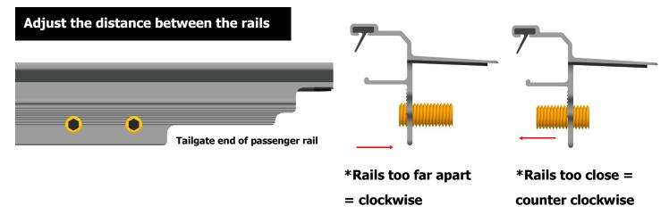
Remove clamp and turn both of the white nylon adjustment screws, using a 1/4" Allen wrench. One complete turn of adjustment screws = 1/16" of adjustment.
