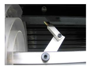
Make sure the threads reach the locking portion of the locknut. If they do not, the jam nut on the back side needs to be retightened. Make sure the joints of the linkages are pointing toward the center of the canister.
