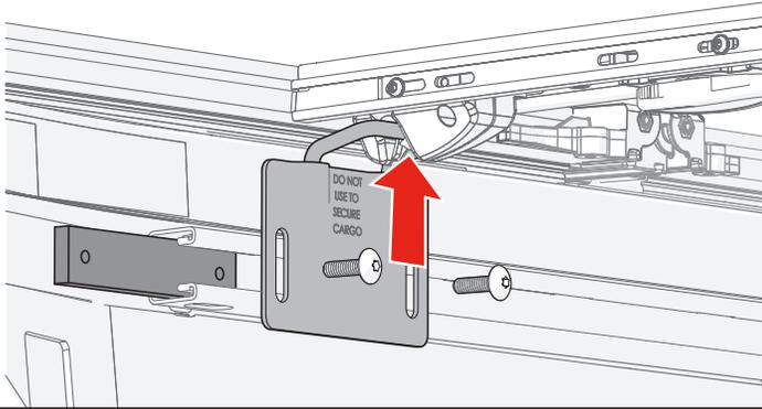
Adjust the rear (tailgate) striker bracket (I) so that it aligns squarely with the cover latch. Push down on cover when tightening the Torx screws (E) so that the rear (tailgate) striker bracket (I) pulls the cover down tightly to the truck bed cap. Do this for both sides of the truck bed.
