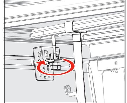
**7** The tether comes assembled on the cab bow of the bed cover. Unscrew the knob from the slide block and separate the block, knob and washer.
