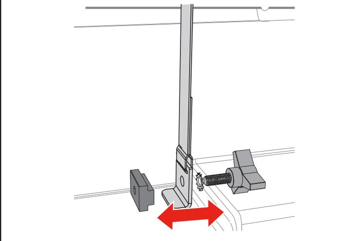
**8** Reassemble the tether by threading the knob through the washer and into the slide block. Install the tether on both sides of the bed.
