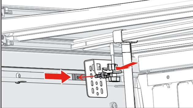
**6** Hook the cab clamp under the cab clamp bracket (C) and tighten the T-handle until it contacts the bracket (C), then tighten two more turns. Do this for both sides of the truck bed.
