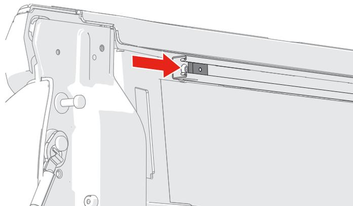
Adjust the rear (tailgate) striker bracket (G) so that it aligns squarely with the cover latch. Push down on cover when tightening the bolt and screws (E) so that the rear (tailgate) striker bracket (G) pulls the cover down tightly to the truck bed cap. Do this for both sides of the truck bed.
