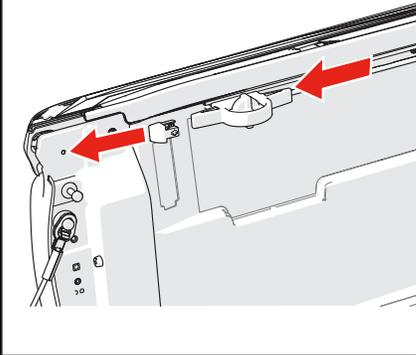
**5** Install the cab slide block (B) into the rear (tailgate) end of the cargo rail. Position near the cab. Align the cab clamp bracket (C) with the cab clamp of the bed cover. Use the Torx screws (D) to mount the cab clamp bracket (C) to the cab slide block (B). Tighten the screws with the T-27 Torx tool. Do this for both sides of the truck bed.
