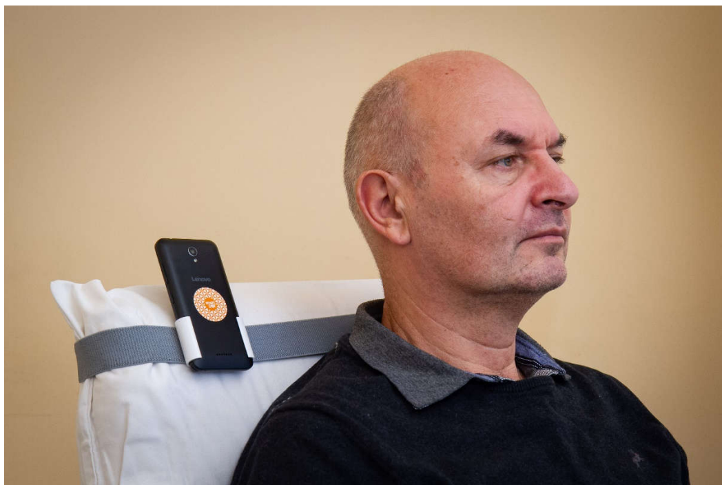
Figure 3: SmartDOT attached to the back of the mobile phone. Mobile phone is located 10 cm from the volunteer's head through the measurement.
