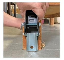
1. Hold the mounting plate up against the leg and allow the silver lever bar to drop down to hang just above the floor. (About 5-1/4" from the floor to the top of the mounting plate).
