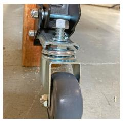
5. Once the plate is attached, put the stem caster up through the bottom of the plate. Put the lock washer in place and then screw the nut in place till hand tightened.
