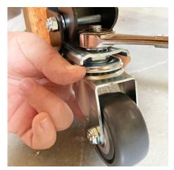
**6.** Use a 3/4" wrench to tighten the nut, grasping the top of the caster to hold it in place until the lock washer has grabbed and you can tighten without having to hold the caster.
