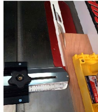
Using a push block or stick, make a rip cut in your material.
