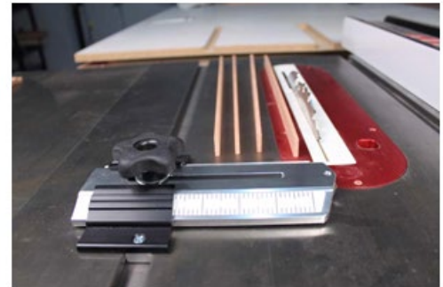
The Thin Rip guide makes it easy to safely and accurately cut thin strips of material on your table saw.
