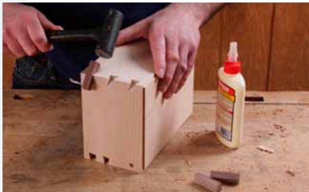
Tapered key leaves no gap. The key slides in from one side only, but the taper guarantees that it fights tightly into the notch.
