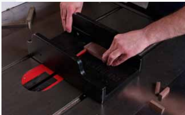
Cut the key. The jig's tablesaw sled is angled slightly to create tapered keys that fit the tapered notches seamlessly. A replaceable throat insert ensures accuracy, safety, and a clean cut.
