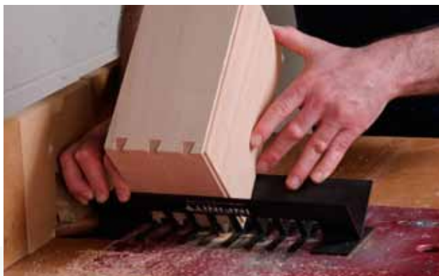
Notch the box. Nestled in the 45° cradle, the box is run through a dovetail bit to create the tapered notches in its corners.
