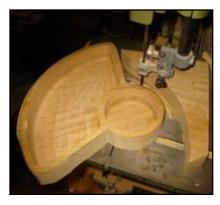
We used our bandsaw to cut away the excess material. Stay on the outside of the perimeter line you made in step #9, sanding will remove the pencil mark.
