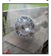
In order to bridge the opening inside your pattern you will need to install a large base plate to your router. We used our 11-3/8" x 11-3/8" Acrylic plate (Item:115-032) which has a center hole large enough to accommodate a bit up to 1-1/4" in diameter. It's important that any plate you use be transparent so that you can see what you are cutting.
