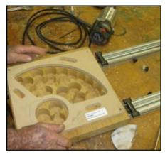
Use the same two predrilled and countersunk holes in the workpiece that you used when laying out your pattern and secure the stock and template to your work surface. We used two of our PROGRIP straight edge clamps (Item: 100-506). These clamps secure to your work surface while safely holding your workpiece at the same time.
