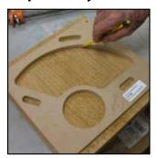
Lightly sand both sides of your material after the glue has finished drying. Choose your template and center it on your material. Use at least two pre-drilled and countersunk screw holes to securely fasten your template to the workpiece. Trace the pattern on your wood and once finished, remove the template.
