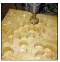
Use a sharp Forstner bit at the drill press to remove the majority of the waste inside the outline of your template. Make sure to leave about 3/16" from the edge of your outline. For tighter corners you may need to use a smaller diameter bit. We used two of our COLT Forstner Bits, 3/4" (Item: 101-123) and 2" (Item: 101-140) diameters.
