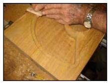
Using your compass (we used a homemade jig) set the desired width of the tray rim. A good rule of thumb is to leave about 1/2" to 5/8" rim width.
