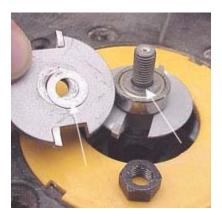
one or two shims between the back cutter and bearing of the rail bit. If the profile sections (decorative cut along the inside edges of all pieces) do not match properly, the stile bit must be adjusted. If the profile area is too loose, add one or two shims between the groove and profile cutter on the stile bit. If the profiles are overly tight, remove one or two shims from between the groove and profile cutter on the stile bit.
