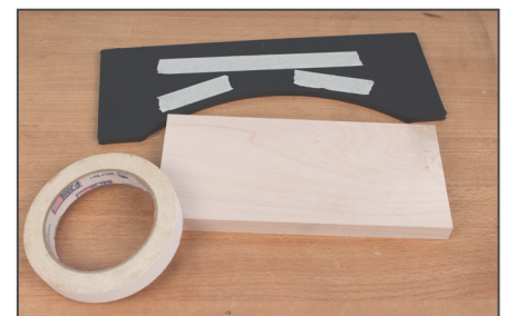
Use plenty of double-sided tape to insure the template does not move during routing!
