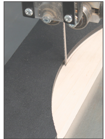
Sawing the waste away very close to the template makes it easier for the flush-trim bit to clean up the edge.
