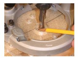
When satisfied with the pivot positions, adjust the pencil so its tip is against the workpiece and draw a full layout circle or ellipse. This lets you be sure that the part can be cut from your blank plus the line is used later to adjust your router for the cut and to trim away excess waste.
