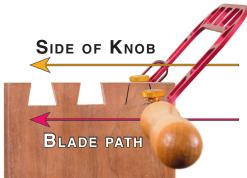
To aid in aiming the saw blade, use the flat sides of the clamping knobs as a reference for where the blade is pointed. The blade always cuts in the same plane as the sides of the knobs. Notice that with most dovetails, you can still see the knob on the forward clamp. This makes it easier to cut straight.
