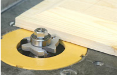
The back cutter bit makes fitting the panel to the stile grooves easy without affecting the presentation face of the raised panel.
