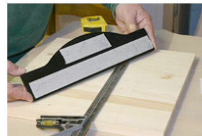
Use plenty of double-sided tape to insure the template does not move during routing!
