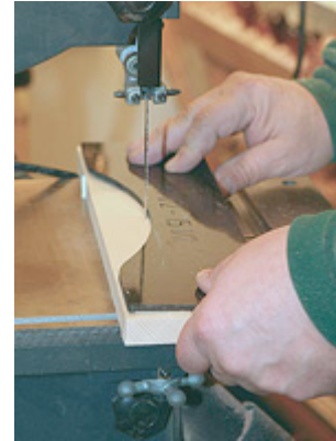
Sawing the waste away very close to the template makes it easier for the flush-trim bit to clean the edge up.
