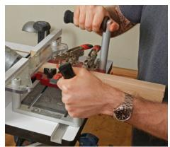
Safe to use. The visor rides against the router table's fence, and its length means there's little chance of the sled and work dangerously pivoting into any fence opening. The two handles keep your hands far from the bit.
