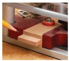
**Tenons too.** The coping sled can also be used for routing tenons, and for molding or shaping workpieces too small to hold safely by hand.
