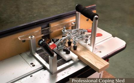
runs the length of the sled and rides against a fence. This keeps the sled square to the router fence and completely away from spinning router bits while maintaining a clear view of the cutting action. However, we have a router table fence in our shop on which a T-track is in the same location as the visor. This could affect the sled's safety execution - but is easily corrected with an auxiliary fence.
