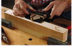
Automatic alignment. The jig straddles a dowel put into the first drilled hole (above), which ensures that the hole in the mating workpiece will be in perfect alignment when drilled using the center bushing (right).
