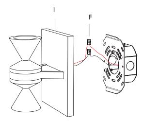
8. Mount the fixture to the wall by wedging the top on the crossbar, then lowering the bottom.
