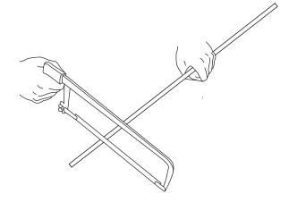
3. Now that the cover tube is cut to 14.75", measure the all thread tube to be 15.25" long. And place a mark, with a marker or tape.
