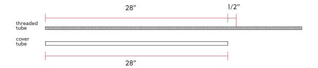
4. Hold down the all thread with a hand or a clamp, use a hacksaw or electrical tool to cut the all thread tube. Recommended to clean all thread tube after cutting to remove any metal chippings.
