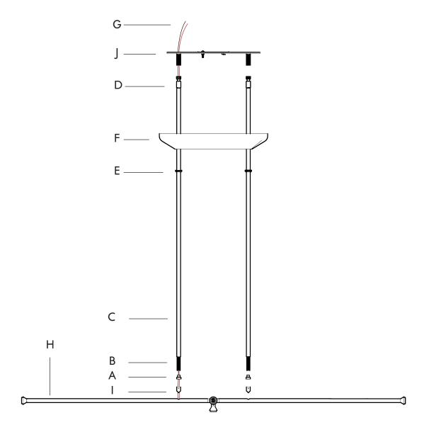
05. Place the crossbar assembly (A) against the two rods and hangstraights (B). Thread the rods (C) down onto the hangstraight until it is flush at the top of the mounting bracket. Secure the stems by threading the two nuts (D)
