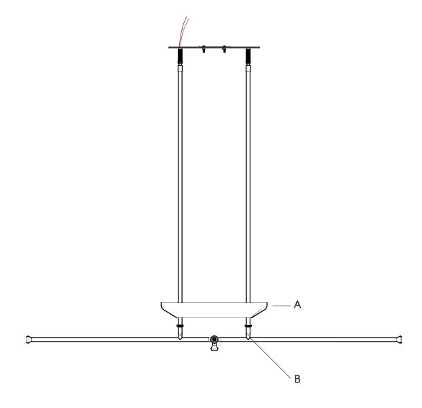
08. Make the electrical connections between the lead AC wires and the driver using the provided Wago Connectors (A)
