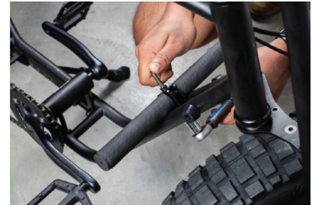
(Fig. 8) Tighten the M6 Nut to 6 Nm .
