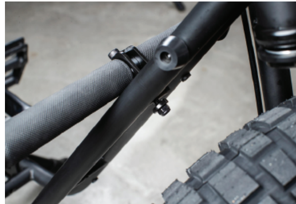
(Fig.7) Washer and M6 Nut.
