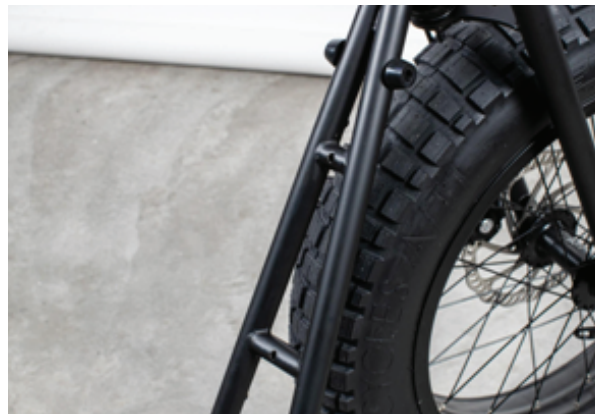
(Fig. 4) The mounting point will be the topmost bar on the down tube.
