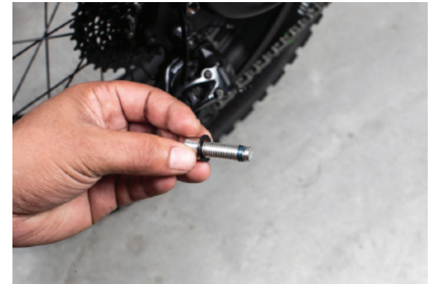
(Fig. 3) Apply the medium strength threadlocker as per the manufacturer's instructions.
