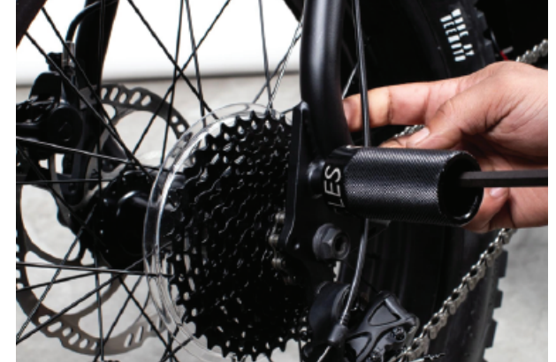
(Fig. 7) Tighten the bolt to 24Nm .
