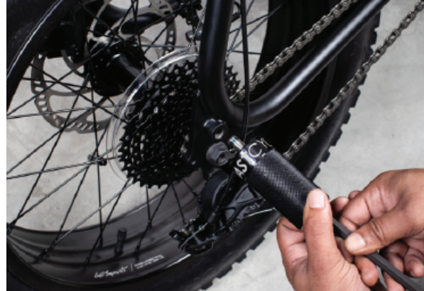
(Fig. 6) Insert the bolt into the foot peg and thread the bolt into the mounting point.
