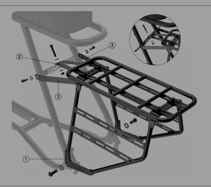
Install rear rack side plate onto the frame dropout mounting point with 2x M10x3mm spacers one on each side first.
