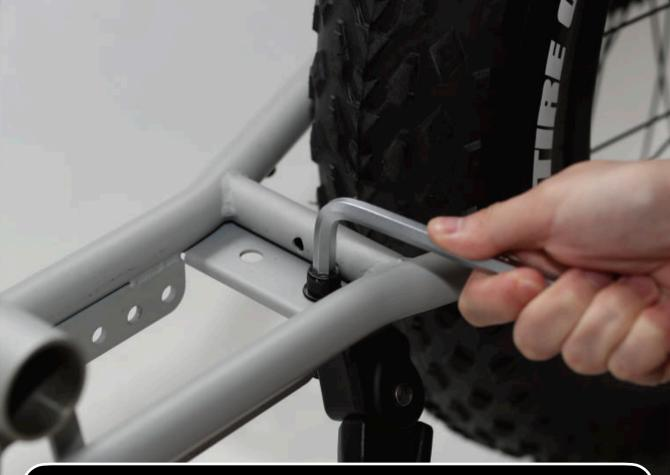
Use a 8.0 (mm) Allen key to tighten the Hex Socket Head Allen Bolt M10 with the mounted Kickstand at the bottom
