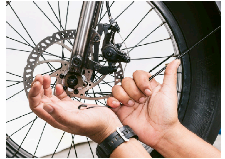
(Fig. 44) Decreasing the bend angle of the strut.
