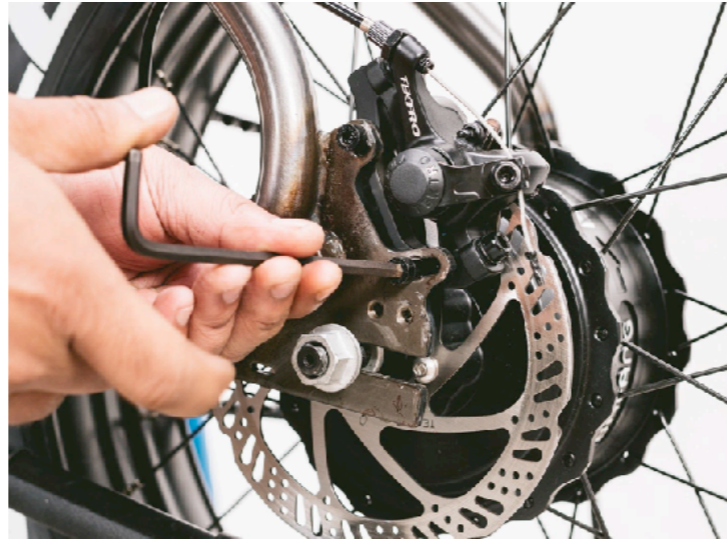
(Fig. 20) Remove the aft most bolt completely.
