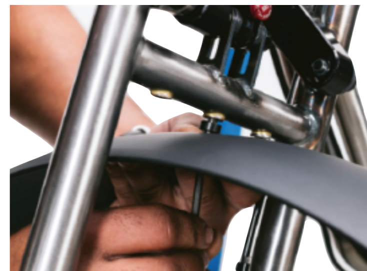
(Fig. 16) Thread the bolt into the middle mounting point on the Buzzwalker fork. Tighten to 4Nm .
