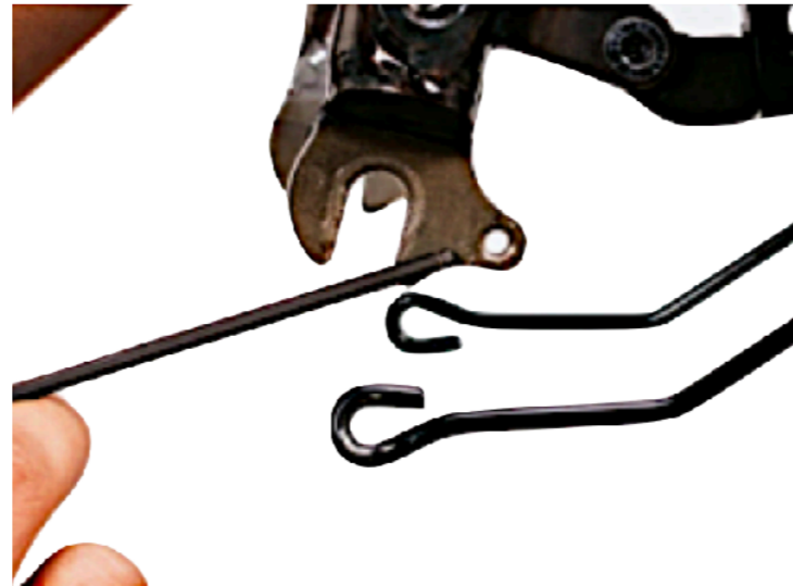
(Fig. 17) Insert the M5x10mm button head bolt through the looped end of the strut and thread the bolt into the threaded hole on the fork dropout.
