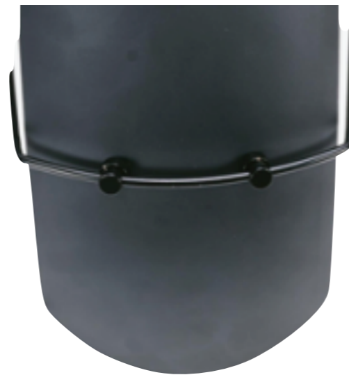
(Fig. 11) Center the struts on the fender.
