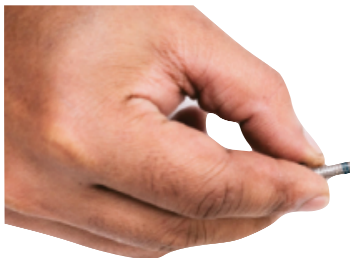
(Fig. 15) Application of the medium strength thread locker to the bolt.
