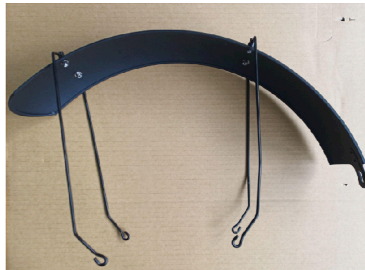
(Fig. 26) Note the orientation of the bend in the struts with relation to the fender.
