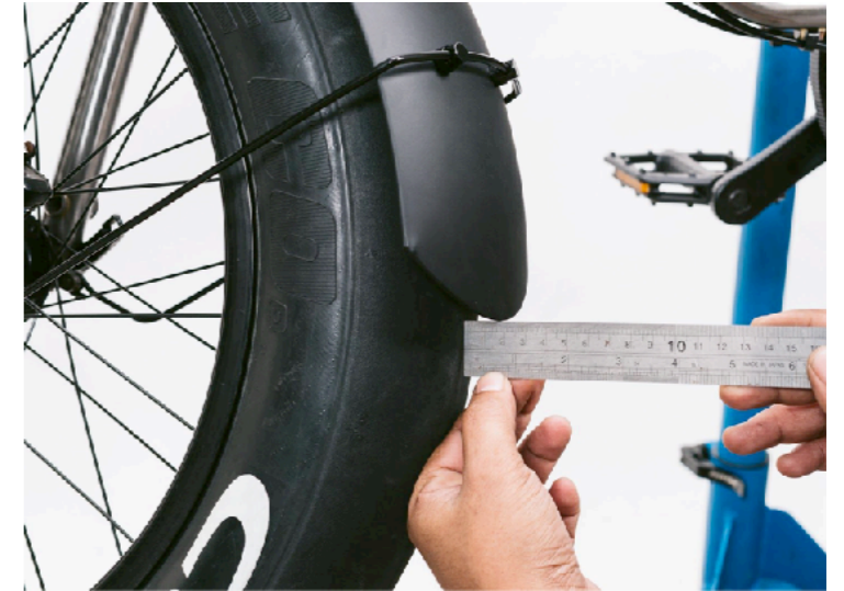
(Fig. 40) Measure the rear edge of the fender to the centreline of the tire.
