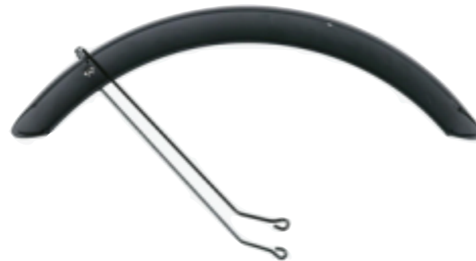
(Fig. 8) Note the orientation of the bend in the struts with relation to the fender.
