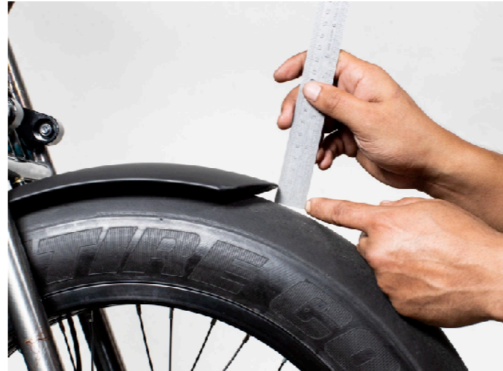
(Fig. 39) Measure the front edge of the fender to the centreline of the tire.
