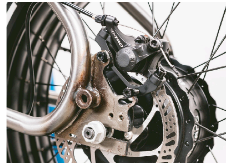
(Fig. 23) Allow the caliper to rest on the frame.
