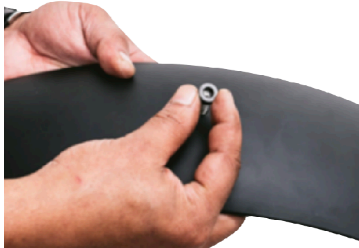
(Fig. 13) Insert the M6x15mm button head bolt from the bottom of the fender.
