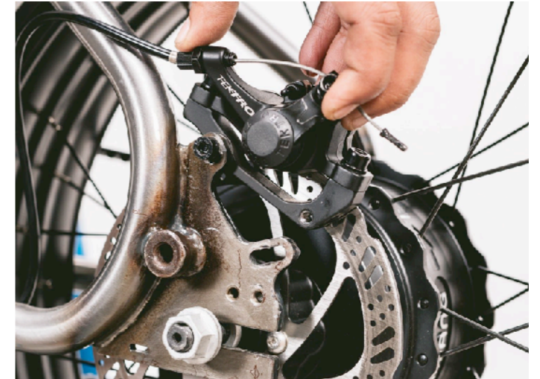
(Fig. 21) Lift the caliper clear of the frame.
