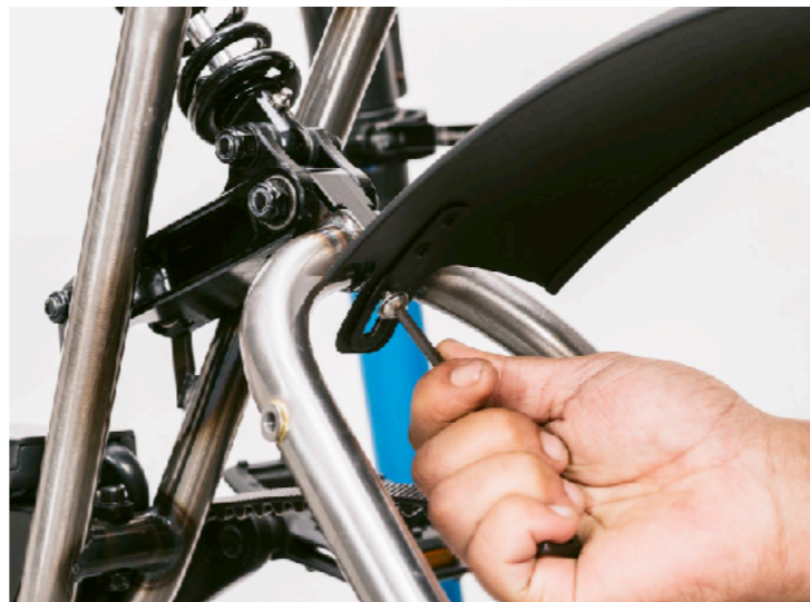
(Fig. 33) Thread the M6 bolt into the hole and tighten to 4Nm . Ensure the fender is as close to the seat stay as possible.
