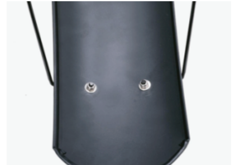
(Fig. 12) Tighten the M5 locknuts to 3Nm .
