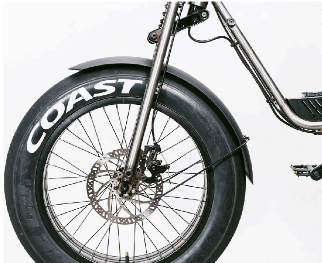
(Fig. 25) Front Fender Installation Complete.
