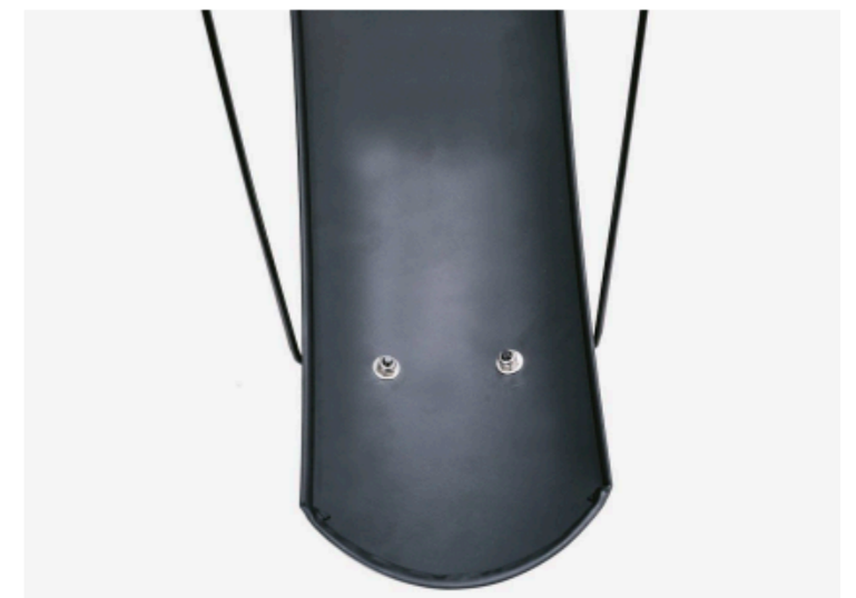
(Fig. 31) Tighten the locknuts to 3Nm .
