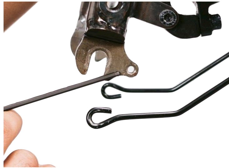
(Fig. 9) Clear the threads of the mounting hole in the fork with a M5x0.8mm tap.
