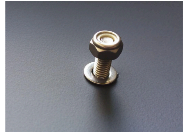
(Fig. 35) Place the M6 washer over the bolt followed by the M6 nylon locknut. Tighten the M6 nylon locknut to 4Nm .
