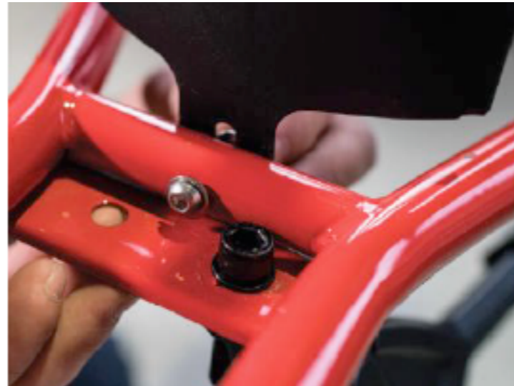
(Fig. 34) Insert the M6x35mm button head bolt with M6 washer into the hole on the chain stay bridge of the frame.
