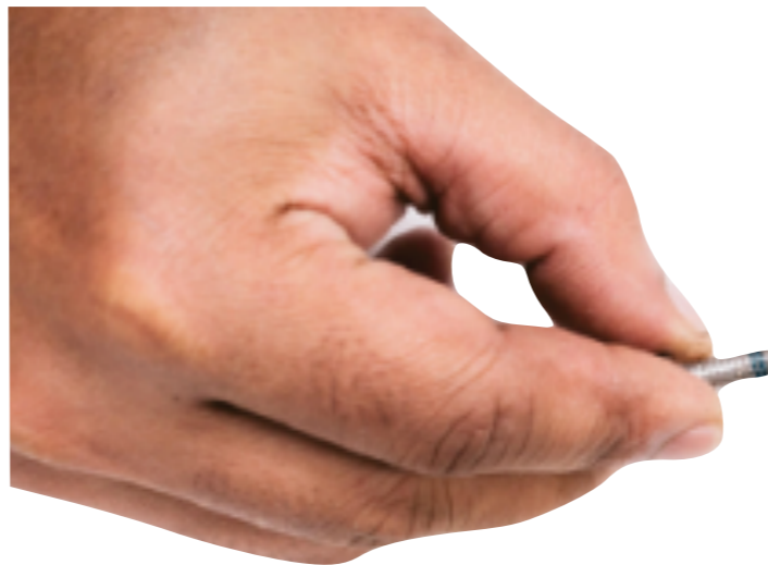
(Fig. 23) Apply medium strength thread locker to the M5x10mm button head bolt.
