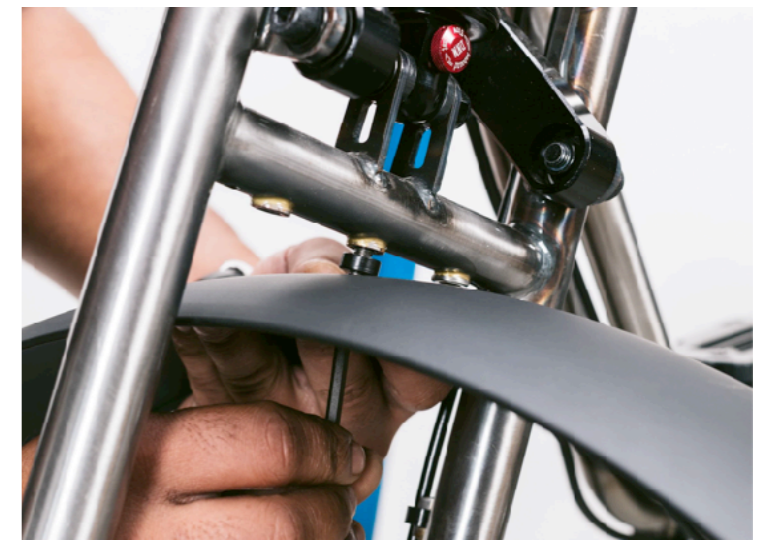
(Fig. 20) Tighten the bolt to 4Nm .
