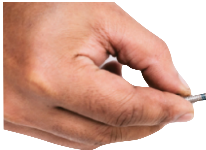
(Fig. 18) Apply Loctite 243 to the bolt threads.
