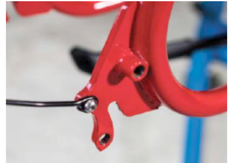
(Fig. 37) Thread the bolt through the fender strut loop and into the mounting point on the rear mounting point. Tighten the bolt to 4Nm .
