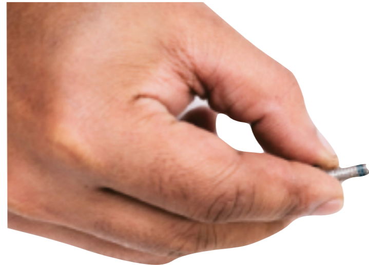
(Fig. 36) Apply medium strength thread locker to the M6x10mm button head bolt.
