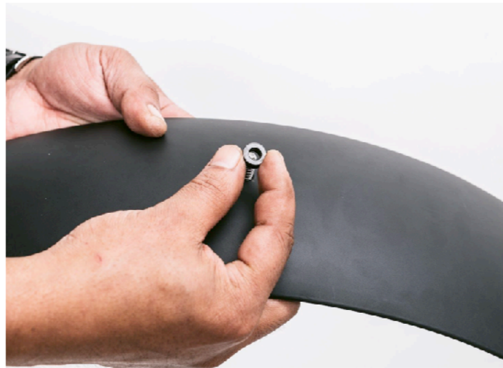
(Fig. 16) Place the M6 washer onto the M6x15mm button head bolt and insert the bolt into the fender from the bottom.
