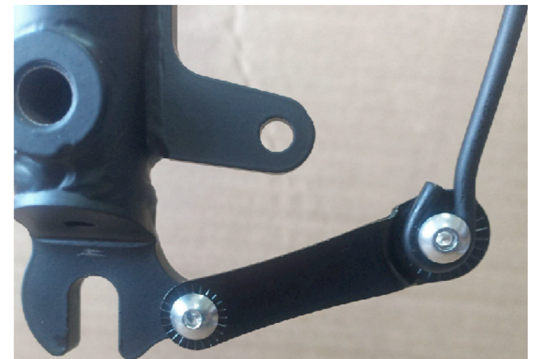
(Fig. 24) Installation on the mounting point on the fork. Tighten to 4Nm .
