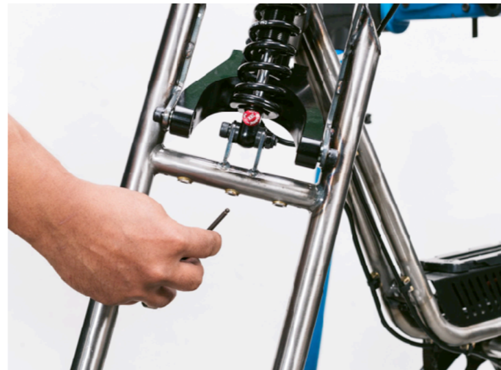
(Fig. 19) Thread the M6x15mm button head bolt into the center mounting point on the Buzzwalker fork.
