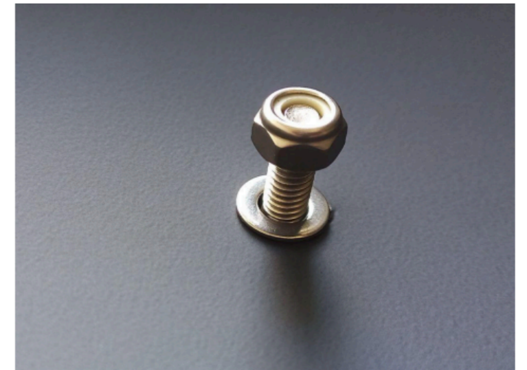
(Fig. 31) Place the M6 washer over the bolt followed by the M6 nylon locknut. Tighten the M6 nylon locknut to 4Nm .
