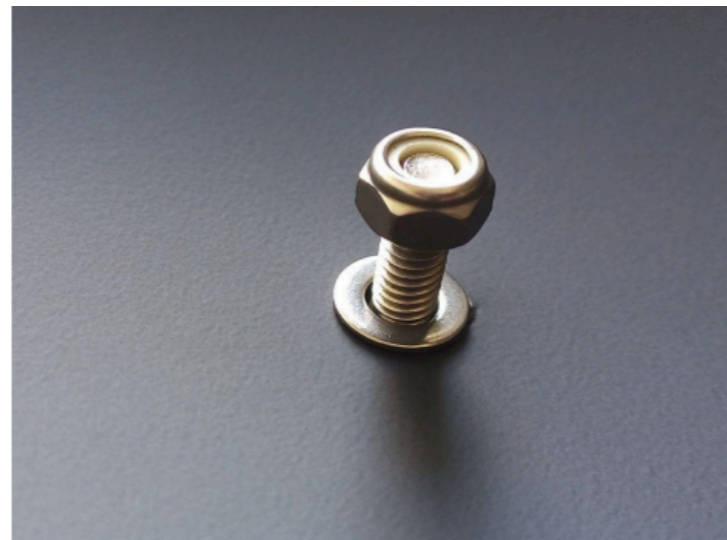
(Fig. 18) Place the M6 washer over the bolt followed by the M6 nylon locknut. Tighten the M6 nylon locknut to 4Nm .
