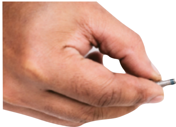
(Fig. 34) Apply medium strength thread locker to the M5x10mm button head bolt.
