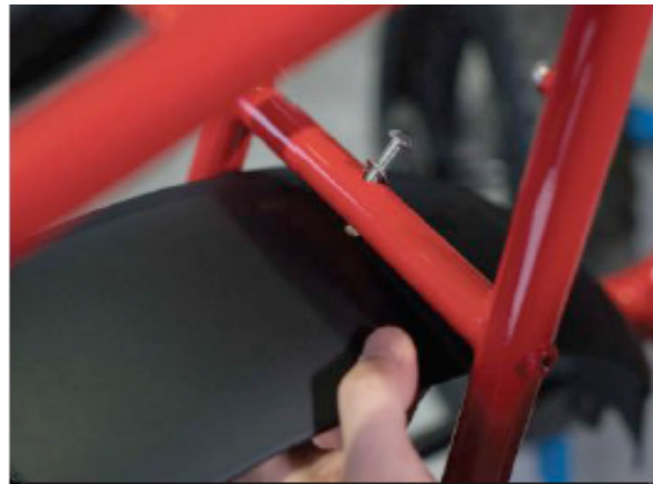
(Fig. 30) Insert the M6x35mm button head bolt with M6 washer into the hole on the seat stay bridge of the frame.
