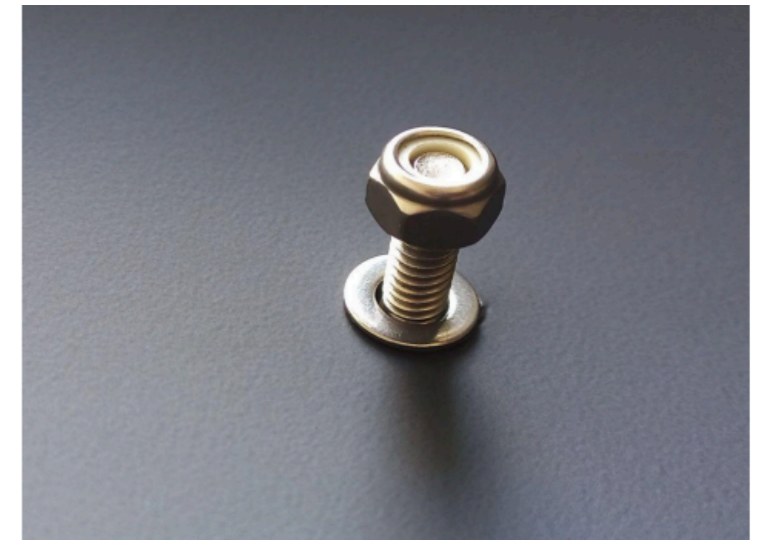
(Fig. 33) Place the M6 washer over the bolt followed by the M6 nylon locknut. Tighten the M6 nylon locknut to 4Nm .
