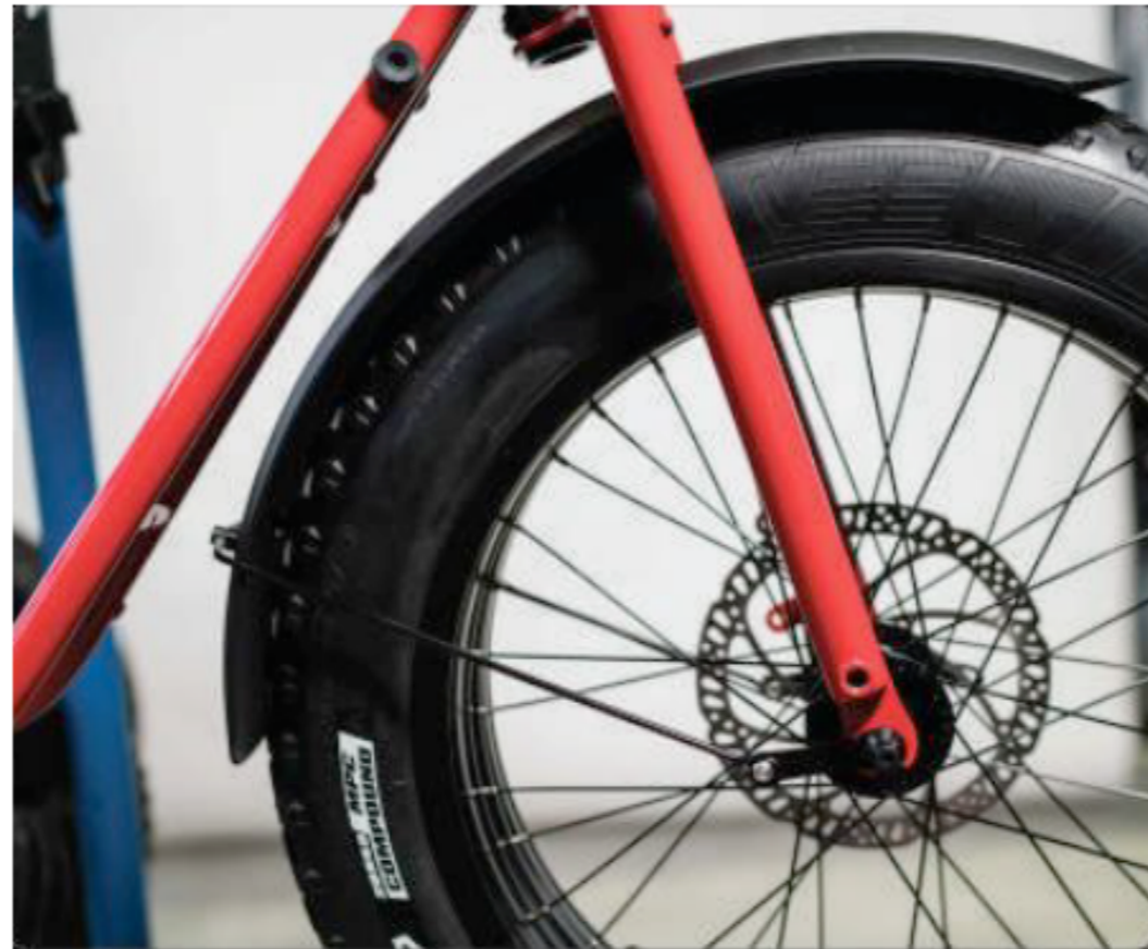
(Fig. 23) Front Fender Installation Complete.
