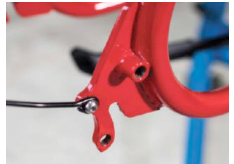
(Fig. 35) Mounting point on the rear of the frame. Tighten the bolt to 4Nm .
