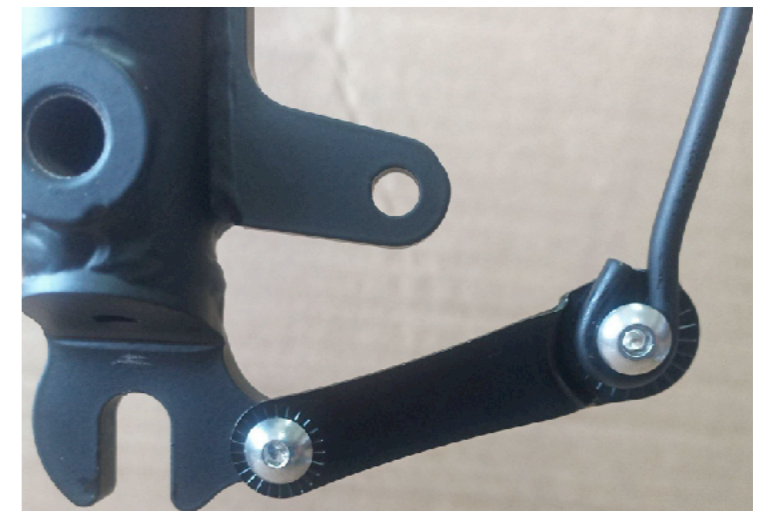
(Fig. 22) Installation on the mounting point on the fork. Tighten the M5 nylon locknut to 4Nm .
