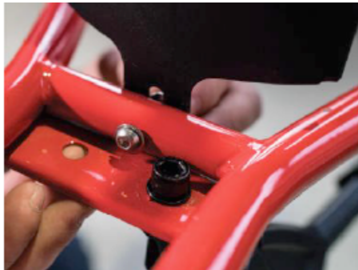
(Fig. 32) Insert the M6x35mm button head bolt with M6 washer into the hole on the chain stay bridge of the frame.
