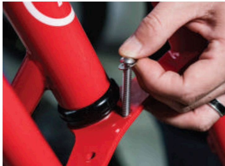
(Fig. 16) Drop the M6x35mm button head bolt with M6 washer through the center mounting point.
