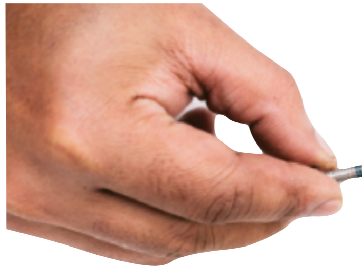
(Fig. 21) Apply medium strength thread locker to the M5x10mm button head bolt.
