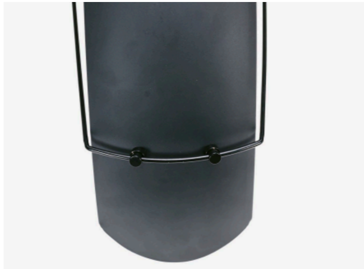
(Fig. 14) Center the struts on the fender.
