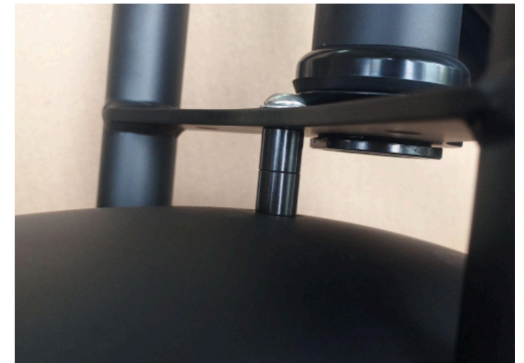
(Fig. 17) Place 2 pieces of M6x10mm spacers over the bolt followed by the fender.
