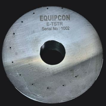
The Ketos Ring is intended to be a quick overall system performance indicator that's used as a total system check for DC magnetic particle equipment. This item is manufactured with subsurface discontinuities which is an excellent tool that provides a quick way to confirm overall performance of your DC output machine.
