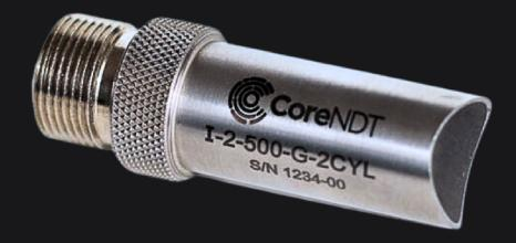
The **Slimline Immersion Transducers** are designed to be watertight and operate underwater. They have an impedance matching layer which helps to allow more sound energy into the water which continues into the part being inspected.
