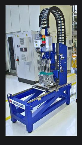
The Sonaflex WTM is an ultrasonic thickness system designed to measure wall thickness on cylinders of combustion engines, even with different metal alloys, during serial production.
