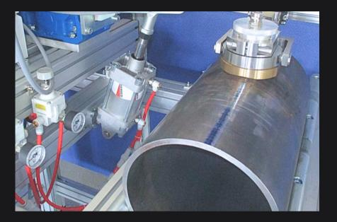
The Sonaflex WSP is EMAT technology that performs in-line inspection of scarfing quality. This system can detect over/under scarfing, tool breakage, or wear alarming the operator when replacement of the tool is required.
