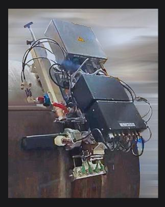
The Sonaflex Weld Robocon accurately follows the weld line via onboard sensors to provide totally wireless and tether-free weld inspection without frames or guides. The scanner is fully self-contained with onboard ultrasonic electronics, a microprocessor, a coolant supply tank, and a drive system to inspect longitudinal or circumferential welds on pipelines or other vessel types.
