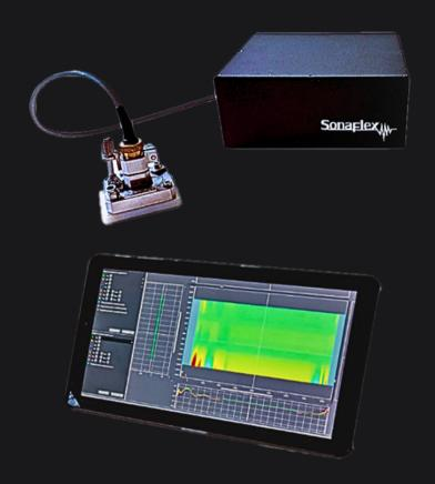
The Sonaflex Mini is a device that consists of a low-profile, battery-operated, compact electronics module and a tablet PC. This system is fully wireless, using Bluetooth and Wi-Fi communication.
