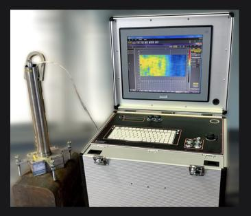
The Sonaflex Liquid Core highlights one of the main advantages of EMAT technology: the absence of water coupling. This makes high-temperature material testing possible. This system allows material temperatures up to 1200°C, which is necessary as the system is intended for the examination of blooms coming directly off the continuous casting line.
