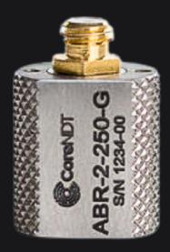
The **Removable Fingertip (Captive Screw) Angle Beams Transducers** are are used in conjunction with a wedge to introduce a refracted shear wave into the material being tested. The standard angle beams are built to be low noise and offer substantial power.
