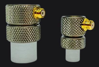
The **Removable Delay Line Transducers** are typically used for thickness gauging and searching for delamination. These transducers use a removable delay line to introduce a time delay into the sound wave. This helps to improve near-surface resolution.
