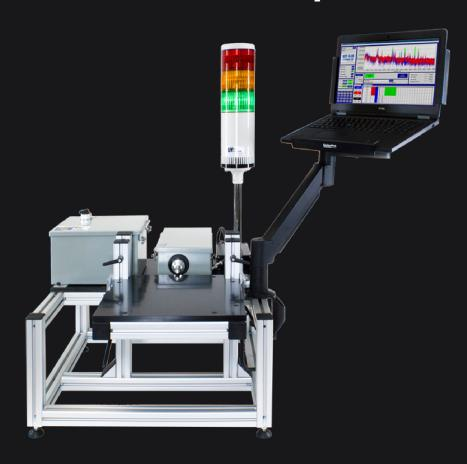
The **RAM-TEST-FIXTURE** is a resonant inspection workstation with an adjustable platform for easy testing of various part sizes and shapes.
