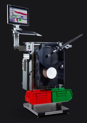
The **RAM-DROP** is a 100% automated fast turnkey inspection system for small parts with automatic sorting of defective parts.
