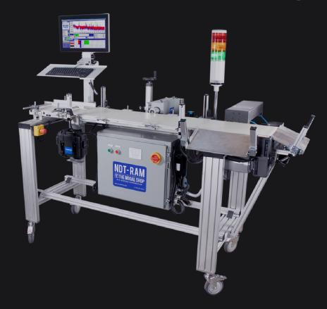
The **RAM-AUTO** is a 100% in-line fully automated turnkey resonant inspection system with an automated conveyor and industrial grade computer that's compatible with a variety of parts.
