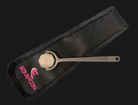
The Equipcon Pie Gauge is a disk of highly permeable material divided into eight sections by non-ferromagnetic material. The joining of sections act as artificial defects that radiate out in different directions from the center which allows the inspector to ensure magnetic fields are properly oriented for the inspection at hand.
