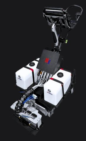
The Sonaflex PL Manual Rider is a manual trolley system with our sophisticated PC-based and flexible Sonaflex platform. It examines the quality of plates and slabs using ultrasonic waves or eddy currents. It detects cracks in both the surfaces of the plate and internal defects, reflecting ultrasonic shear waves propagating in the direction of about 45 degrees to the surfaces.
