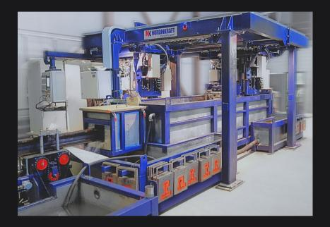
The Nordiscan-Rails is our platform of ultrasonic inspection systems designed for the detection of internal and surface defects in railroad rails, which inspects the head, web, and foot using ultrasonic phased array and EMAT probes. We offer 3 different configurations.
