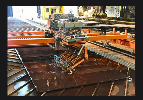
The Nordiscan-PL scanners are intended for fully automated off-line ultrasonic examination of the body and edges of plates, coils, slabs, and ingots. These systems are designed to perform fully automatic, high-performance inspections of flats outside of the production line on a charging table.
