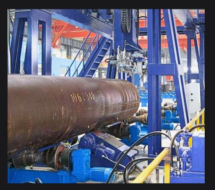
The Nordiscan-PI is our common platform for all tube and pipe inspection applications. Modular design allows the use of UT (piezo), phased array, UT arrays, EC, and EMAT technology depending on the specific tasks needed for our clients.
