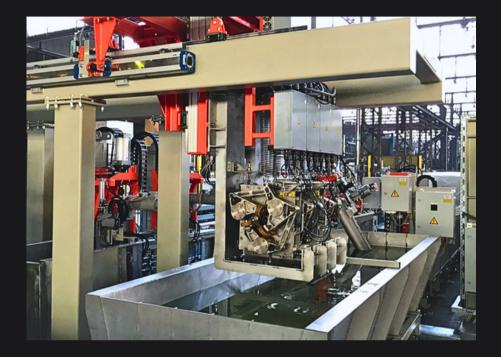
The Nordiscan-BB systems are intended for the examination of bars, billets, and other more complex profiles. Offered in 2 different configurations.
